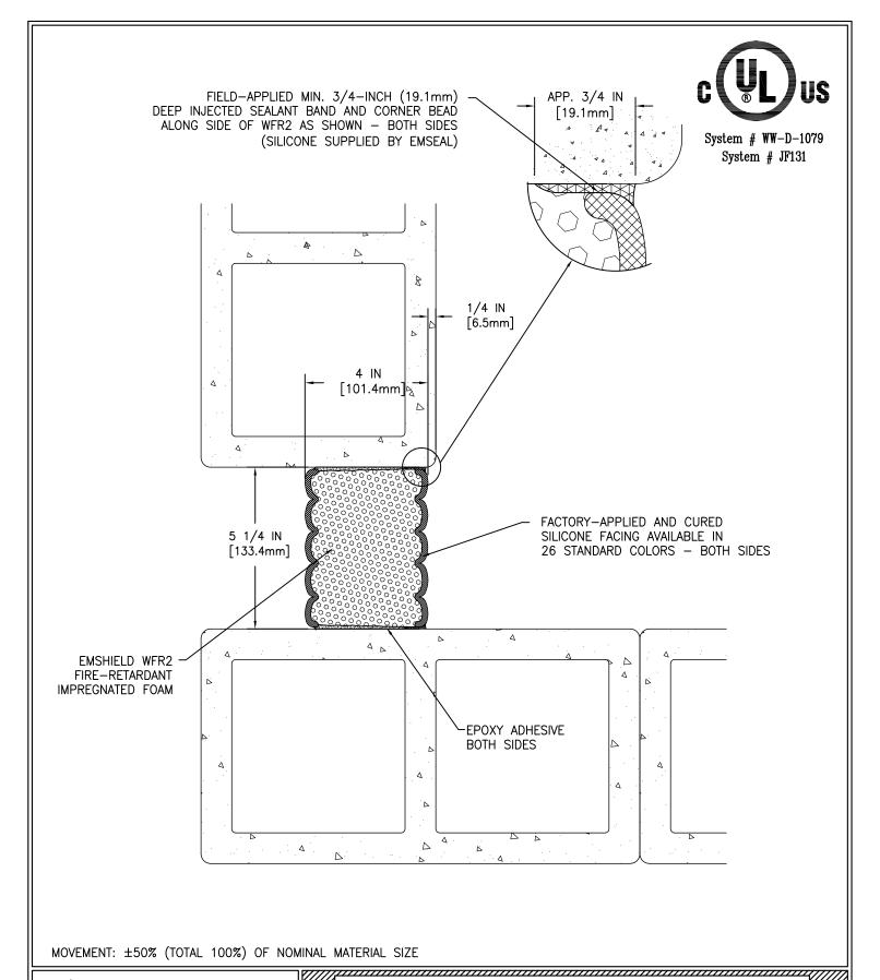
EMSEAL'S EMSHIELD WFR2 HAS BEEN TESTED IN ACCORDANCE WITH UL 2079 IN THE CONFIGURATION DEPICTED IN SYSTEM # WW-D-1079. USE OF THIS MATERIAL IN WALL ASSEMBLY CONFIGURATIONS OTHER THAT DEPICTED IN UL SYSTEM # WW-D-1079 WILL NOT ENCUMBER OR LOWER THE RESISTANCE OF THE WALL BUT IS DONE SO AT THE DESIGNERS' DISCRETION AND RESPONSIBILITY FOR DESIGN OF A FIRE RATED WALL ASSEMBLY THAT MEETS APPLICABLE STANDARDS FOR THE PROJECT AND WHICH ADDITIONALLY IS CAPABLE OF RESISTING THE APPROXIMATELY 2.5 PSI
