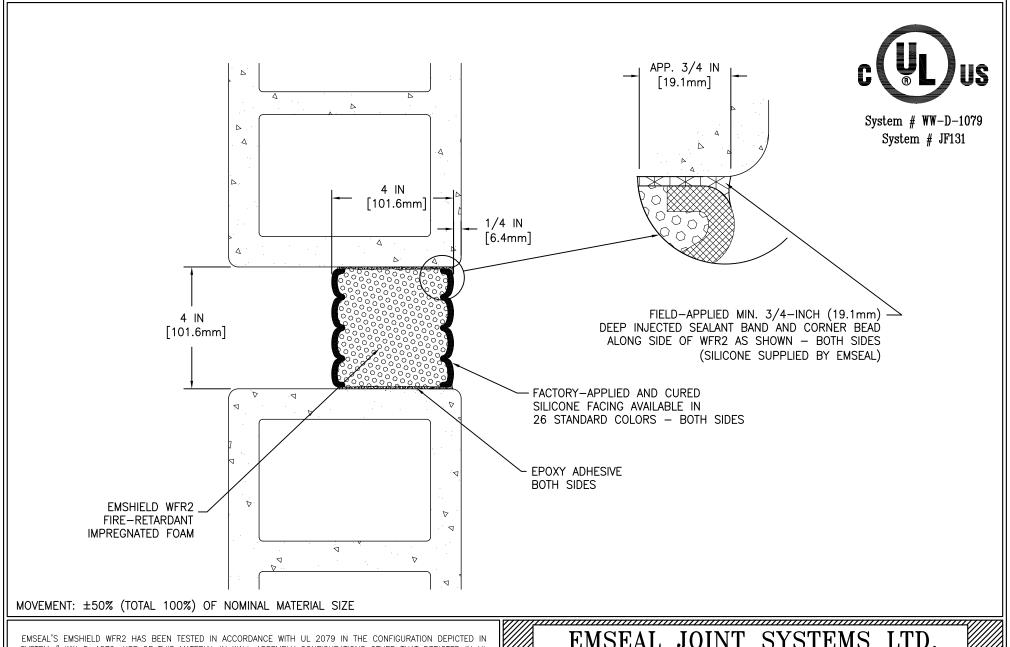
SYSTEM # WW-D-1079. USE OF THIS MATERIAL IN WALL ASSEMBLY CONFIGURATIONS OTHER THAT DEPICTED IN UL SYSTEM # WW-D-1079 WILL NOT ENCUMBER OR LOWER THE RESISTANCE OF THE WALL BUT IS DONE SO AT THE DESIGNERS' DISCRETION AND RESPONSIBILITY FOR DESIGN OF A FIRE RATED WALL ASSEMBLY THAT MEETS APPLICABLE STANDARDS FOR THE PROJECT AND WHICH ADDITIONALLY IS CAPABLE OF RESISTING THE APPROXIMATELY 2.5 PSI (120 LBS PER FOOT OF JOINT BASED ON 4-INCH DEPTH OF SEAL) BACKPRESURE OF THE WFR2 MATERIAL.
