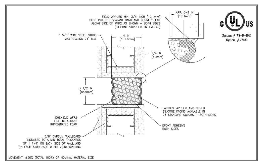
EMSEAL'S EMSHIELD WFR2 HAS BEEN TESTED IN ACCORDANCE WITH UL 2079 IN THE CONFIGURATION DEPICTED IN SYSTEM # WW-D-1081. USE OF THIS MATERIAL IN WALL ASSEMBLY CONFIGURATIONS OTHER THAT DEPICTED IN UL
