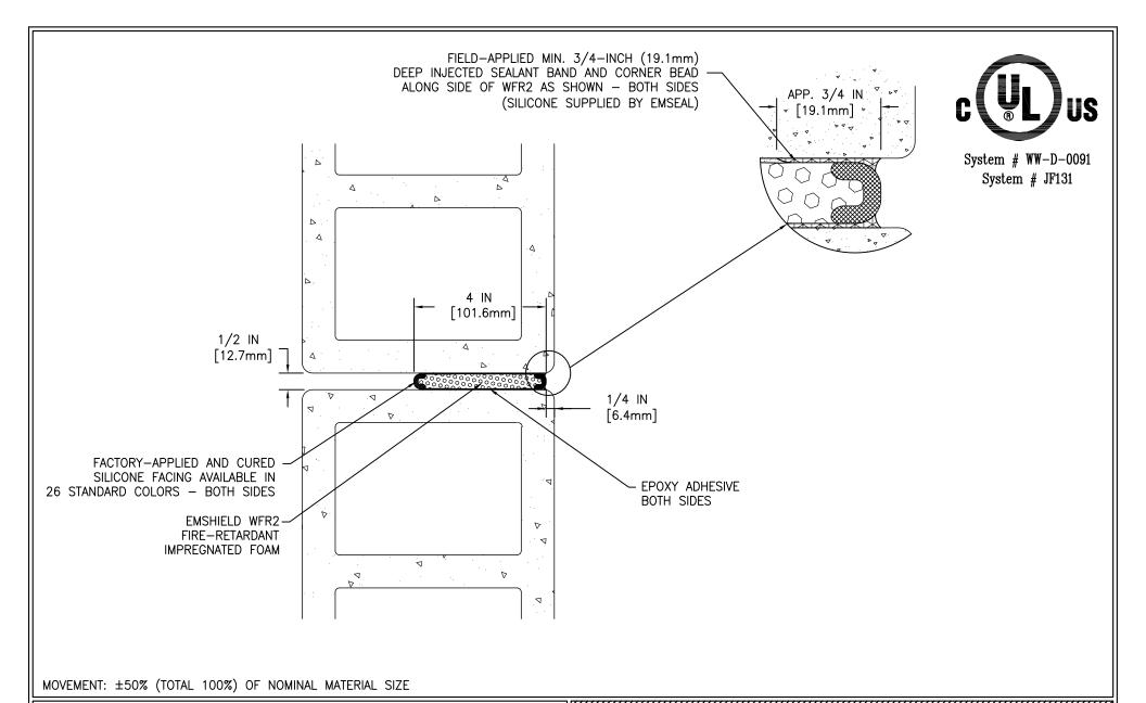
EMSEAL'S EMSHIELD WFR2 HAS BEEN TESTED IN ACCORDANCE WITH UL 2079 IN THE CONFIGURATION DEPICTED IN SYSTEM # WW-D-0091. USE OF THIS MATERIAL IN WALL ASSEMBLY CONFIGURATIONS OTHER THAT DEPICTED IN UL SYSTEM # WW-D-0091 WILL NOT ENCUMBER OR LOWER THE RESISTANCE OF THE WALL BUT IS DONE SO AT THE DESIGNERS' DISCRETION AND RESPONSIBILITY FOR DESIGN OF A FIRE RATED WALL ASSEMBLY THAT MEETS APPLICABLE STANDARDS FOR THE PROJECT AND WHICH ADDITIONALLY IS CAPABLE OF RESISTING THE APPROXIMATELY 2.5 PSI
