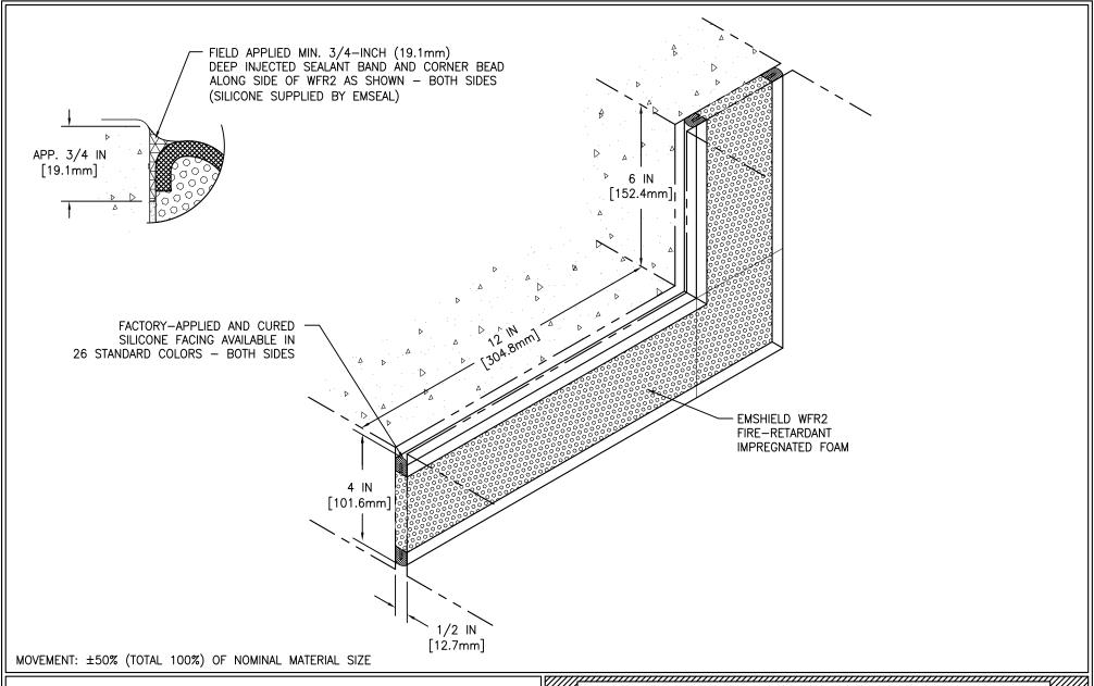
EMSEAL'S EMSHIELD WFR2 HAS BEEN TESTED IN ACCORDANCE WITH UL 2079 IN THE CONFIGURATION DEPICTED IN SYSTEM # WW-D-0091. USE OF THIS MATERIAL IN WALL ASSEMBLY CONFIGURATIONS OTHER THAT DEPICTED IN UL SYSTEM # WW-D-0091 WILL NOT ENCUMBER OR LOWER THE RESISTANCE OF THE WALL BUT IS DONE SO AT THE DESIGNERS' DISCRETION AND RESPONSIBILITY FOR DESIGN OF A FIRE RATED WALL ASSEMBLY THAT MEETS APPLICABLE STANDARDS FOR THE PROJECT AND WHICH ADDITIONALLY IS CAPABLE OF RESISTING THE APPROXIMATELY 2.5 PSI
