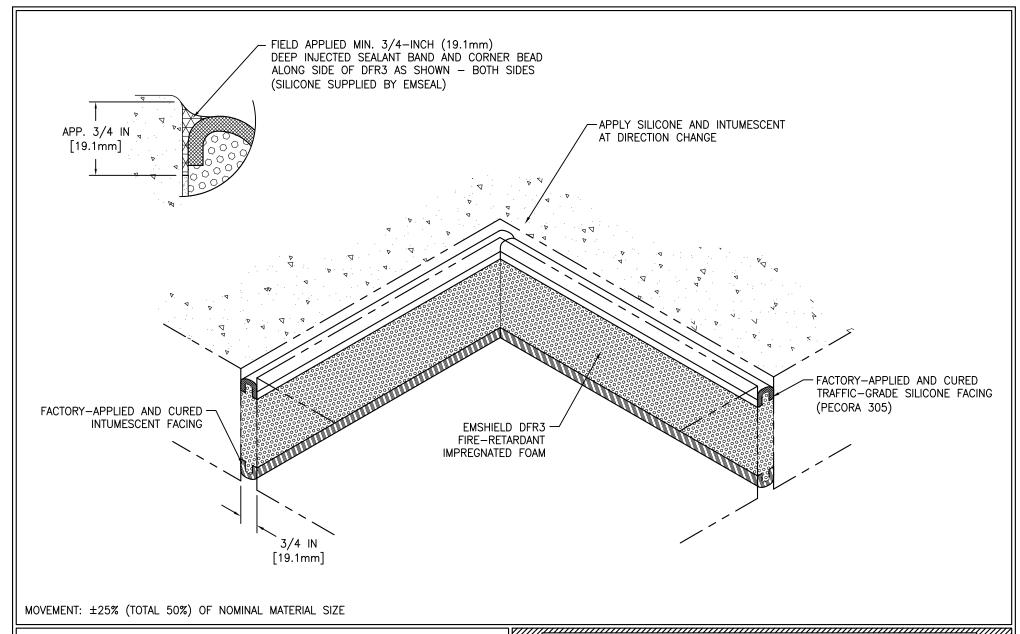
EMSEAL'S EMSHIELD DFR3 HAS BEEN TESTED IN ACCORDANCE WITH UL 2079 IN THE CONFIGURATION DEPICTED IN SYSTEM # FF-D-0078. USE OF THIS MATERIAL IN WALL ASSEMBLY CONFIGURATIONS OTHER THAT DEPICTED IN UL SYSTEM # FF-D-0078 WILL NOT ENCUMBER OR LOWER THE RESISTANCE OF THE WALL BUT IS DONE SO AT THE DESIGNERS' DISCRETION AND RESPONSIBILITY FOR DESIGN OF A FIRE RATED WALL ASSEMBLY THAT MEETS APPLICABLE STANDARDS FOR THE PROJECT AND WHICH ADDITIONALLY IS CAPABLE OF RESISTING THE APPROXIMATELY 2.5 PSI
