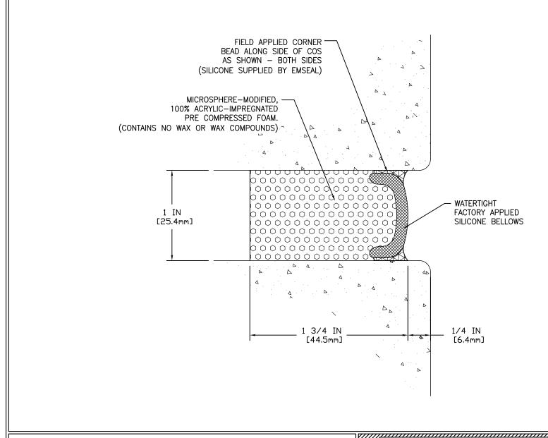
MOVEMENT: ±50% + 1/2 IN (13mm) - 1/2 IN (13mm)
