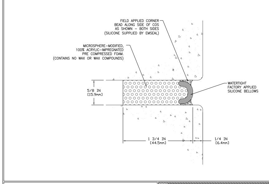
MOVEMENT: ±50% + 5/16 IN (8mm) - 5/16 IN (8mm)
