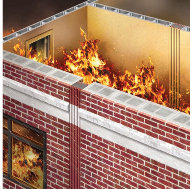
Fire-resistance-rated expansion joints help keep fire in the compartment of origin. - EMSEAL Photo
