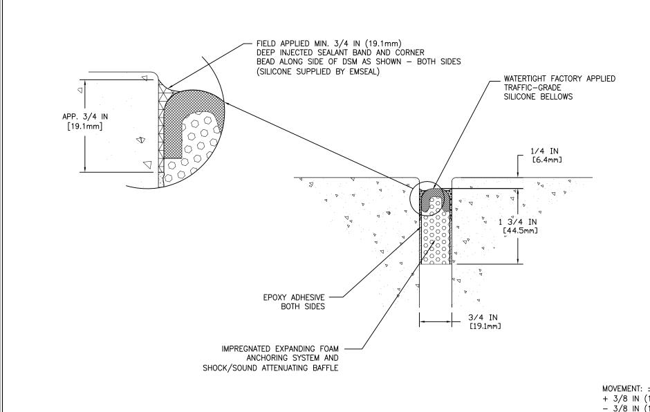
MOVEMENT: ±50% + 3/8 IN (10mm) -3/8 IN (10mm)
