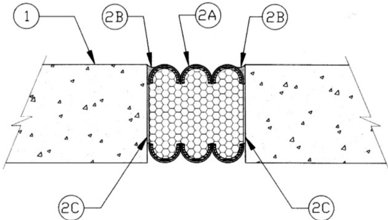
1. **Wall Assembly** — Min 5 in. (127 mm) thick reinforced lightweight or normal weight (100-150 pcf, or 1600-2400 kg/cu meter), structural concrete. Wall may also be constructed of any UL Classified **Concrete Blocks\***.
