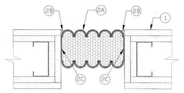
1. **Wall Assembly** — The 2 hr fire rated framed gypsum wallboard wall assembly shall be constructed of the materials and in the manner specified in the individual U300 or U400 Series Wall and Partition Designs in the UL Fire Resistance Directory and shall include the following construction features:
