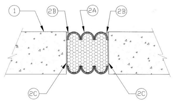
1. **Wall Assembly** — Min 4 in. (100 mm) thick reinforced lightweight or normal weight (100-150 pcf, or 1600-2400 kg/cu meter), structural concrete. Wall may also be constructed of any UL Classified **Concrete Blocks\***.
