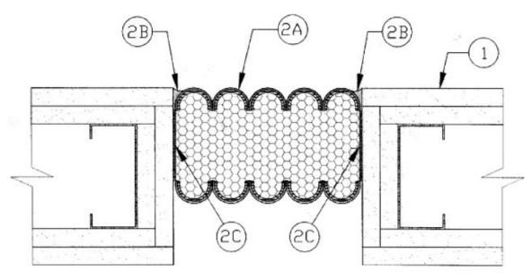
1. **Wall Assembly** — The 2 hr fire rated framed gypsum wallboard wall assembly shall be constructed of the materials and in the manner specified in the individual U300 or U400 Series Wall and Partition Designs in the UL Fire Resistance Directory and shall include the following construction features:
