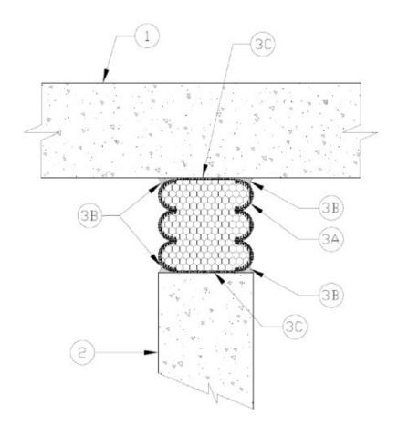
1. Floor Assembly — Min 4-1/2 in. (114 mm) thick reinforced normal weight 150 pcf, (2400 kg/m<sup>3</sup>), structural concrete.
