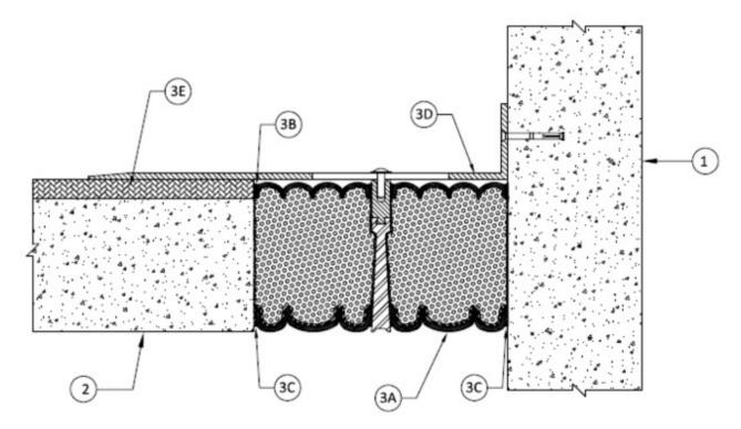
1. Wall Assembly — Min 6 in. (150 mm) thick reinforced normal weight or lightweight (100-150 pcf, or 1600-2400 kg/cu meter) structural concrete. Wall may also be constructed of any UL Classified Concrete Blocks\*.
