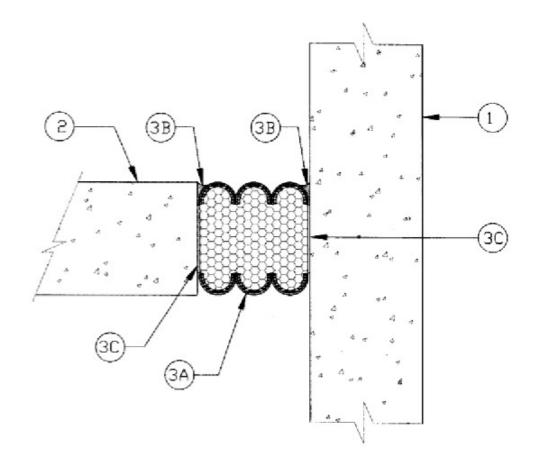
1. Wall Assembly — Min 4-1/2 in. (114 mm) thick reinforced normal weight 150 pcf, (2400 kg/cu meter) structural concrete. Wall may also be constructed of any UL Classified Concrete Blocks\*.
