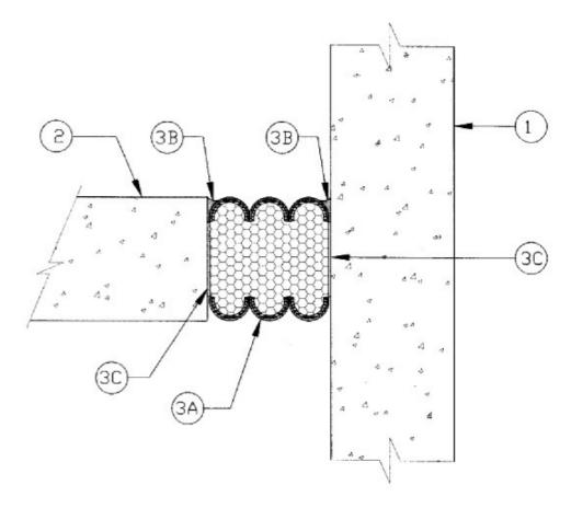
1. **Wall Assembly** — Min 4-1/2 in. (114 mm) thick reinforced normal weight 150 pcf, (2400 kg/cu meter ) structural concrete. Wall may also be constructed of any UL Classified **Concrete Blocks\*.**
