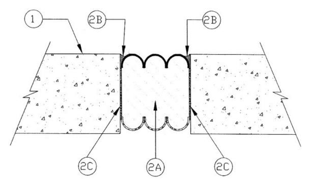
1. Floor Assembly — Min 4-1/2 in. (114 mm) thick reinforced normal weight 150 pcf, (2400 kg/cu meter), structural concrete.
