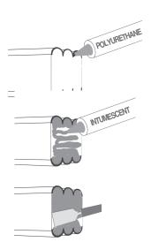
IMPORTANT: All sticks of SSF2 foam MUST have a coating of intumescent on the faces of all joins. This ensures that joins do compromise the fire barrier.
