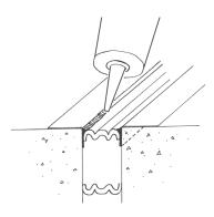
Where SecuritySeal SSF2 foam meets at butt joins, tool the excess polyurethane that squeezes out from the top and between the bellows.
