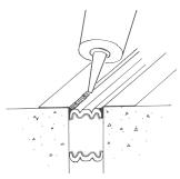
IMPORTANT: Silicone left between the wrinkles of the bellows could constrain movement — using a caulk knife, remove excess sealant and blend what remains into the bellows.
