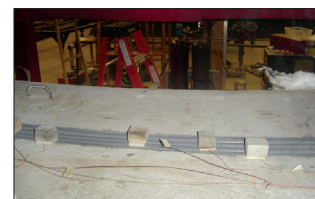
Thermocouples register no more than 248°F (120°C)
