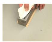
Lightly, quickly and thoroughly wipe the cured silicone facing with a lint-free rag made damp with water to remove the release agent.
