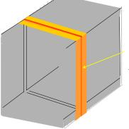
In this typical tunnel application, BG is used under the slab and up the blind-side formed walls. At the transition above the blind-side walls, BG wraps over the roof in softscapes or joins to MIGUTAN on the freestanding walls and across the roof or plaza deck in hardscape wear courses.
