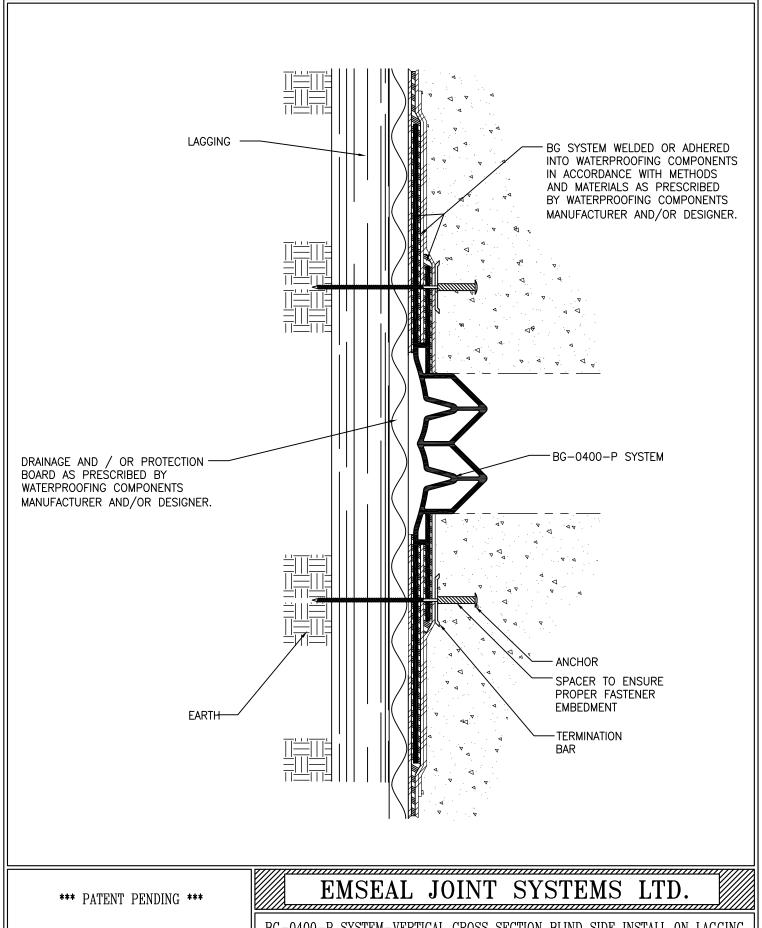
BG-0400-P SYSTEM-VERTICAL CROSS SECTION BLIND SIDE INSTALL ON LAGGING
