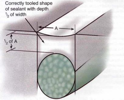
Proper positioning of a backer rod and the tooling of liquid sealant, to achieve a functional joint.
