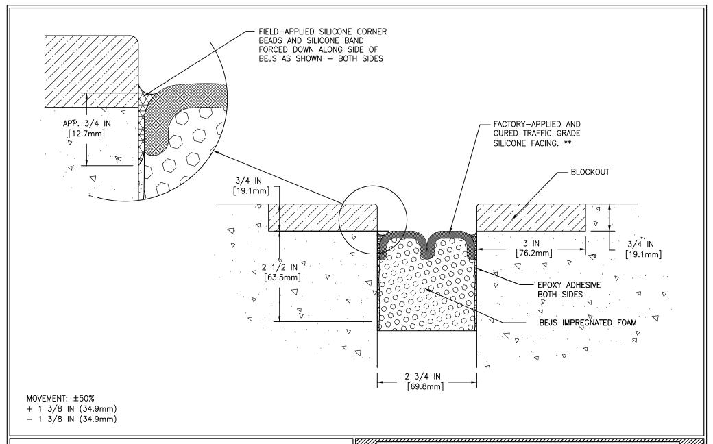
\*\* WIDTHS UNDER 1 1/4 -INCH (32mm) HAVE A CONVEX SINGLE-BELLOWS SURFACE. WIDTHS FROM 1 1/2 -INCH (39mm) TO 4-INCHES (100mm) HAVE A DUAL-BELLOWS SURFACE.
