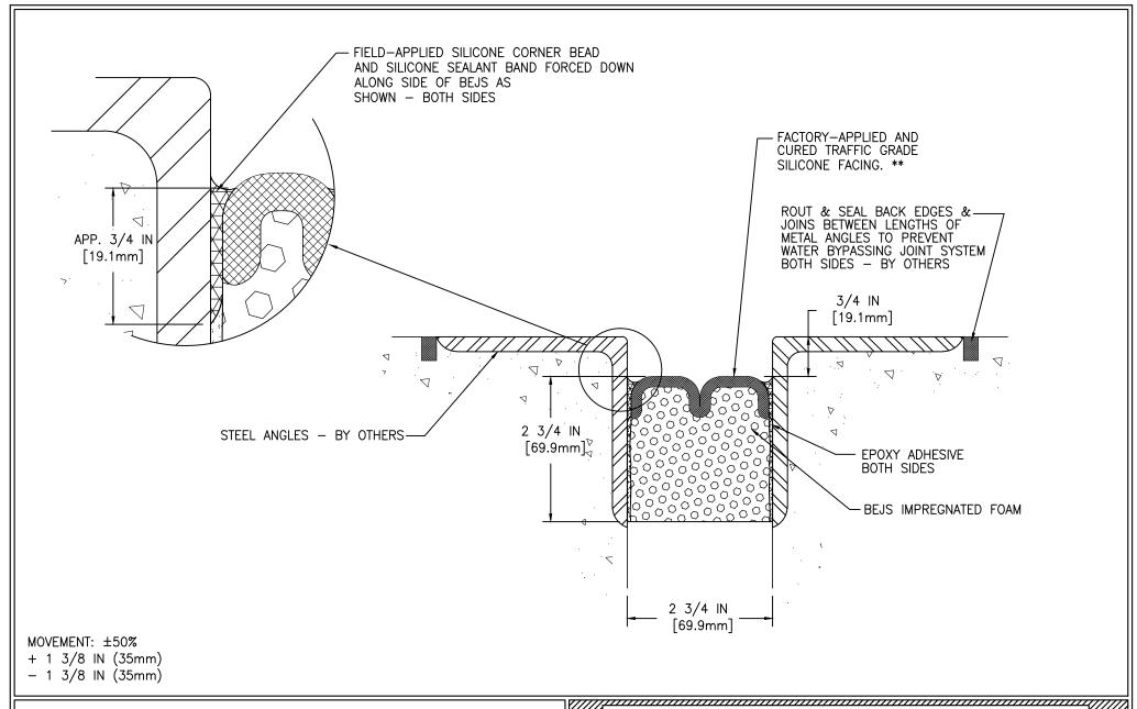
\*\* WIDTHS UNDER 1 1/4 -INCH (25mm) HAVE A CONVEX SINGLE-BELLOWS SURFACE. WIDTHS FROM 1 1/2 -INCH (25mm) TO 4-INCHES (100mm) HAVE A DUAL-BELLOWS SURFACE.
